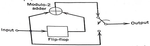
Q10.Figure shows the encoder for a rate ½ constraint length K=4 convolutional code. Determine the encoder output produced by the message sequence 10111...
